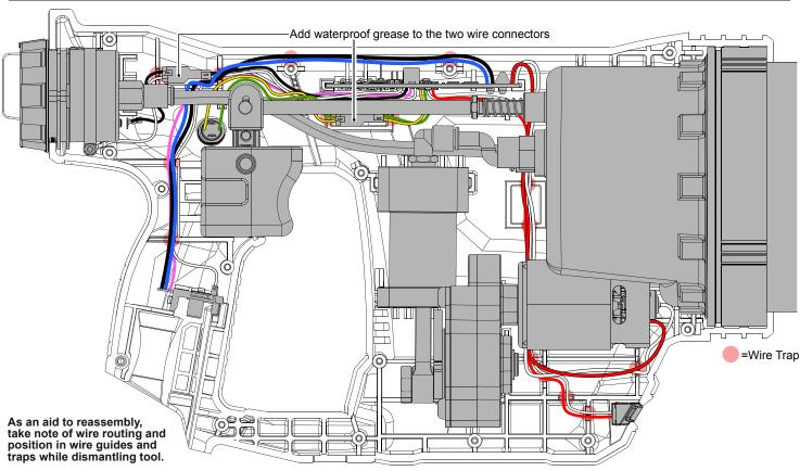
Be careful and avoid pinching wires between handle halves when reassembling. Be sure all mechanical components are firmly and squarely seated in housing support (left housing halve). Be sure all wires are tucked completely down in wire traps and that there is no interference prior to installing housing cover (right housing halve). Check for proper functionality of trigger and pressure gauge dial. Install battery and make sure tool operates properly.
